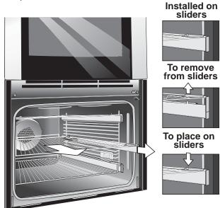
Pull oven rack forward and lift it up off the oven rack slider.
